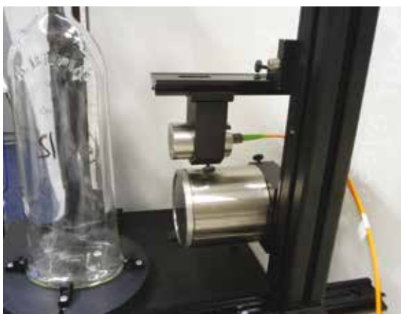
Figure 1: 12mm and 15mm probe stacked for a measurement comparison on an oval bottle. See also table 1 for 12mm and 15mm data.
