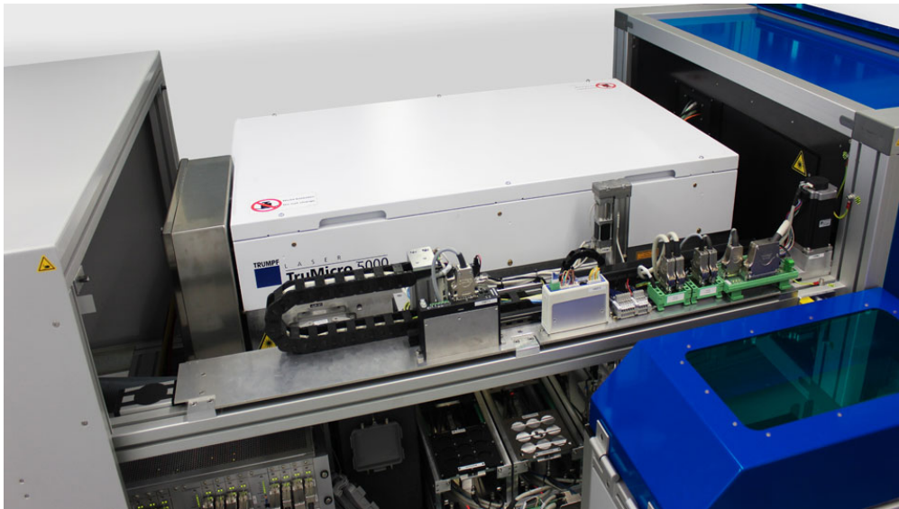
The engine of the laser depaneler: the ultrashort pulse laser by TRUMPF with 30 W and 150 \mu s pulse power. Photo | ic-automation
