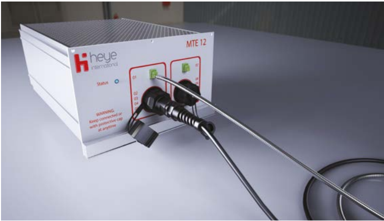
Multi-point measurement system with chromatic confocal sensor for measuring the wall thickness of glass containers. A single-point sensor is shown in the background in the right-hand image (images: Heye International).
