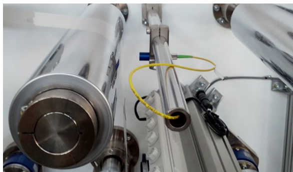
Measuring the thickness of multilayer plastic foils
